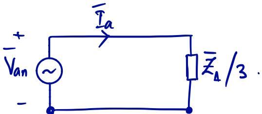
Then, the load is the per-phase equivalent
