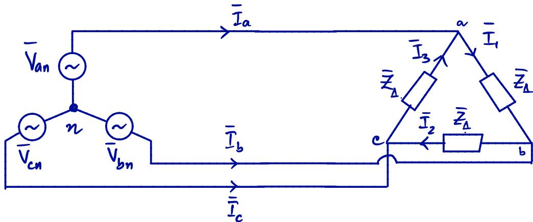
Let us transform the  $\Delta$ -load to an equivalent Y-load. To simplify,
